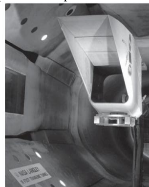
Fig 15:- The SAMPSON inlet cowl as installed in the NASA Langley Transonic Wind Tunnel
