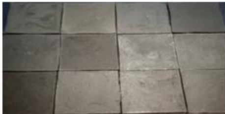
Figure 4. PET plastic roof tiles samples
