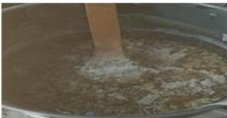
Figure 3 : Melted PET wastes mixed with sand
