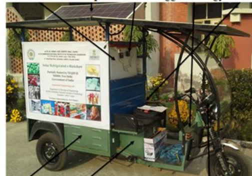
Battery bank MPPT-controller Battery indicator
