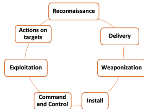
Fig. 2 A Cyber Kill Chain model advanced attack stages.
