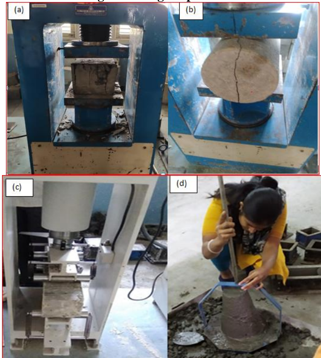
Fig.4. Tests setup: (a) compressive st., (b) splitting tensile st., (c) flexural st., and (d) Slump test.
