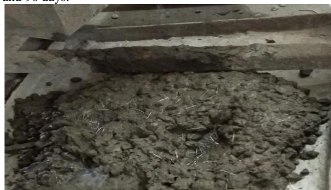
Fig.2 Blending of rubber treated concrete with hook end steel filaments
