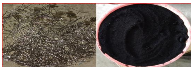
Fig.1. Hooked end steel filaments and 30 mesh crumb rubber
