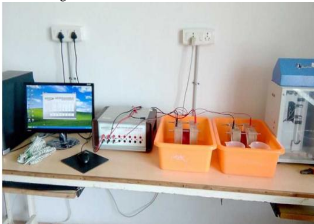
Figure 6.7 Test setup for RCPT
