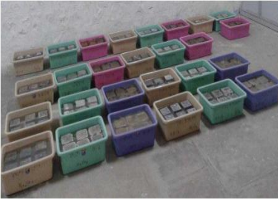
Figure 6.4 Specimens immersed in 5% H 2 SO 4 and 5% HCl solutions
