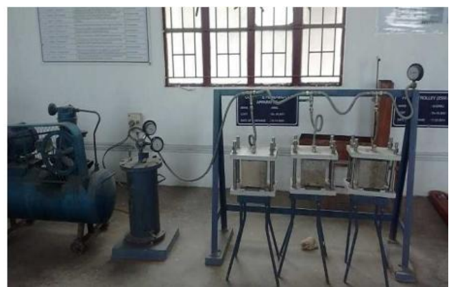
Figure 6.2 Water permeability test set-up
