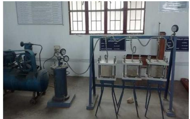
Figure 6.2 Water permeability test set-up
