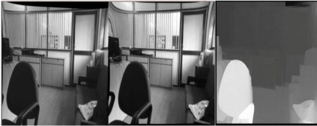
Figure 8 : Stereo images with calculated disparity
