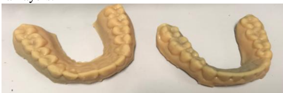
Figure 1. Dental mold produced by Fused Deposition Modelling method
