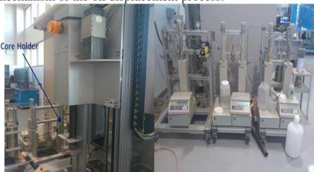
Figure 3. A photograph of the core flooding system.
