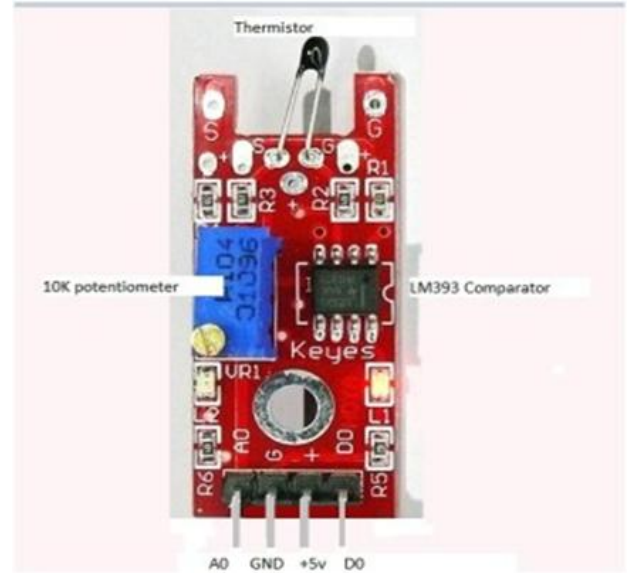
Fig. 2. Temperature Sensor
