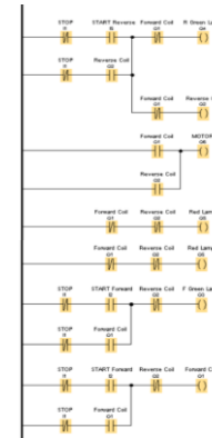
Fig 4. Control Circuit of the Forward- Reverse Simulation
