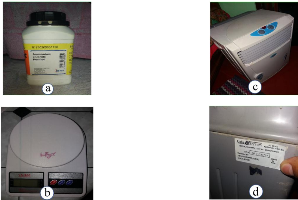
Fig. 7: Some experimental components (a) \text{NH}_4\text{Cl} salt (b) Weight measuring instrument (c) DEC (d) Specifications of DEC.
