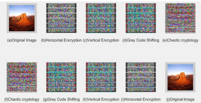
Fig.7 a) Original image of Desert b) Horizontal encoded, c) Vertical encoded, d) Gray-code shifting e) Encoded image after Chaotic cryptography f) Chaotic cryptography encoded image g) Decoded image (gray-code shifting) h)Vertically decoded image i) Horizontally decoded image and j) Decoded original image
