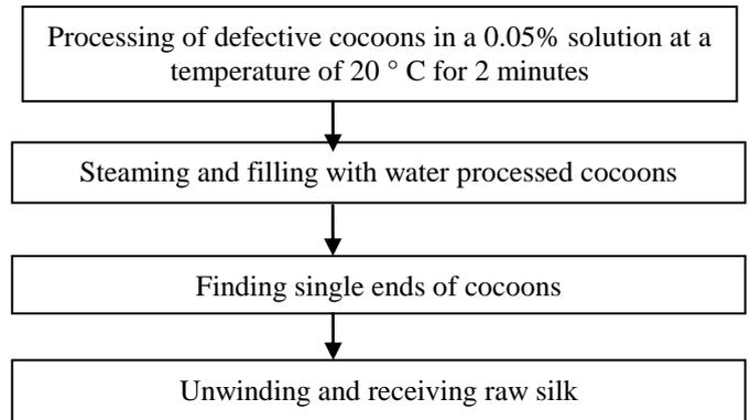
Processing defective cocoons before unwinding leads to an increase in the speed of unwinding and an increase in the yield of raw silk by 5-10%. The unwinding speed is an important factor when unwinding cocoons. In our studies, we determined the dependence of the breakage of silk on the speed of unwinding. The results are shown in (Table 4).
