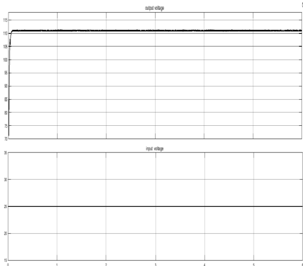
Fig.7 Output and input Voltages in open loop condition
