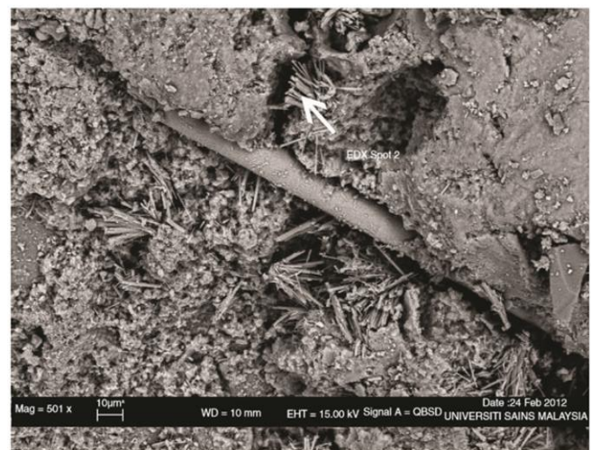
Fig. 1 SEM image (5000× magnification) of the 2.4% glass fiber in tropical air for 18 months [16].
