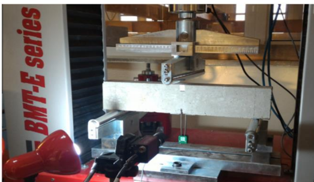
Fig. 3 Bending test set-up [58]
