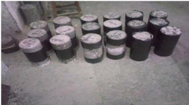
Fig. 13 Wrapped specimens with CFRP [94].
