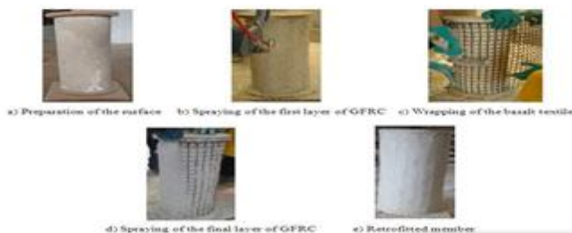
Fig. 14 Retrofitting process of the members [95]
