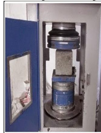
Fig .4 Compression test on concrete cube
