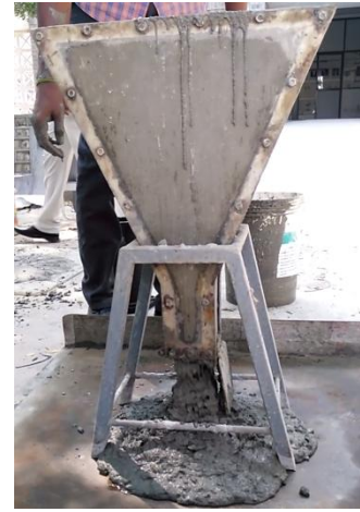
Fig .3 V funnel test
