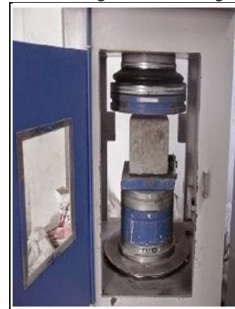
Fig .4 Compression test on concrete cube
