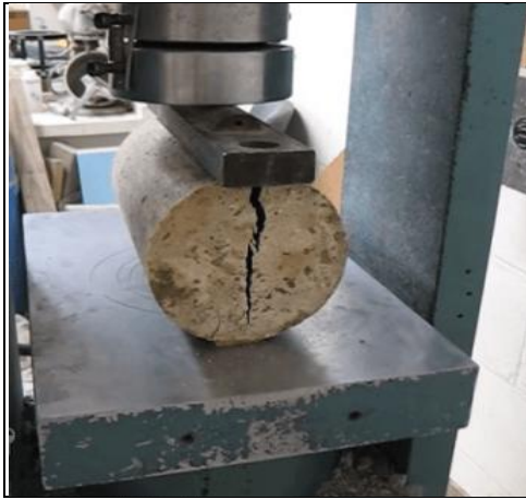
Fig. 5 Split tensile strength test on cylinder
