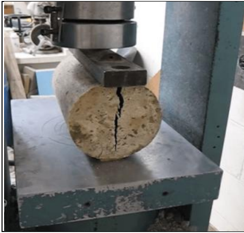
Fig.5 Split tensile strength test on cylinder
