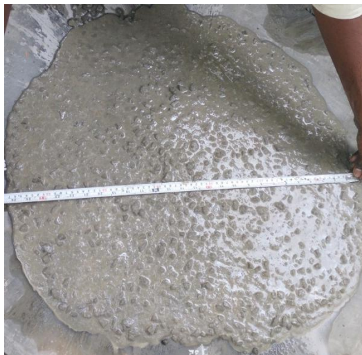
Fig .2 Slump test
