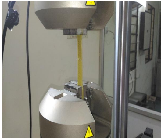
Fig. 3. UTS test on Servo Dynamic Hydraulic Universal Testing Machine
