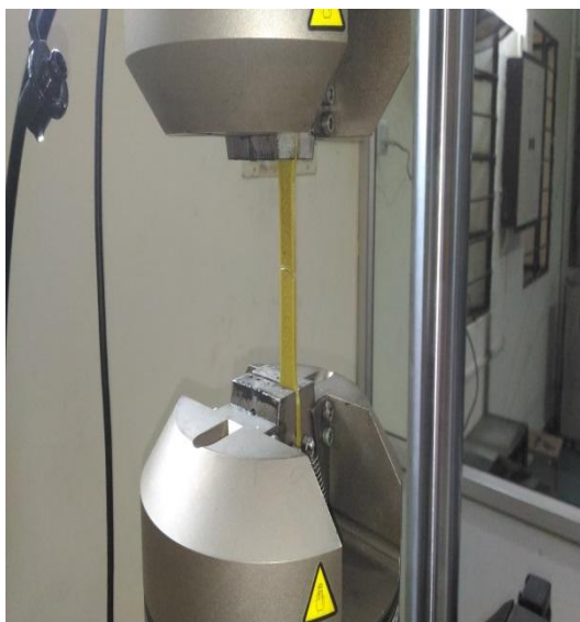
Fig. 3. UTS test on Servo Dynamic Hydraulic Universal Testing Machine
