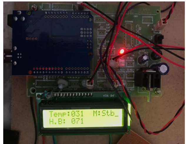
Figure10: Output of LCD when patient is stable, temperature and pulse rate are normal
