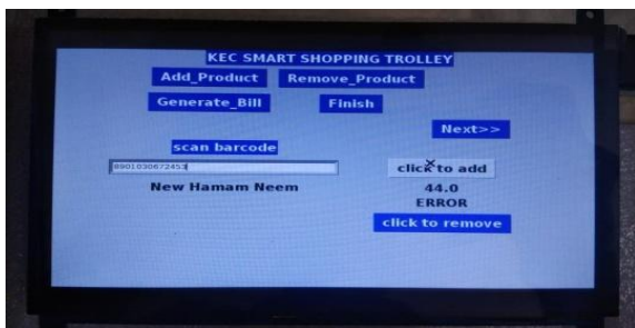
Fig. 6. Theft detection displayed as error on display
