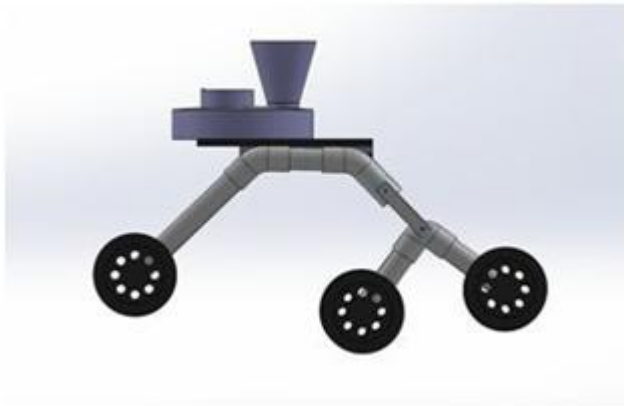
Figure 13: Solid Works Side View 3d Models Of Rocker Bogie System
