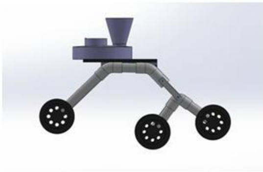
Figure 13: Solid Works Side View 3d Models Of Rocker Bogie System
