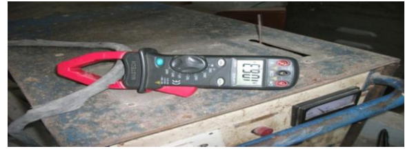
Figure 3: Current Measurement by Clamp-meter
