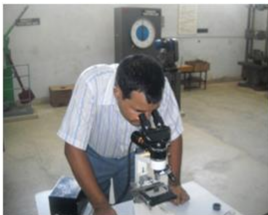
Figure 2: Measurements of Weld Bead Dimensions with Metallurgical Microscope
