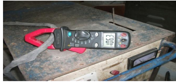
Figure 3: Current Measurement by Clamp-meter
