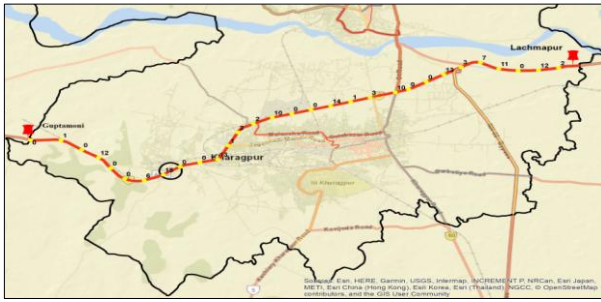
Fig.10: Black spot identification: (a) NH-6 (c) NH-60 (e) OT road (NH-60), Total accident each KM distance: (b) NH-6 (d) NH-60 (f) OT road (NH-60).
