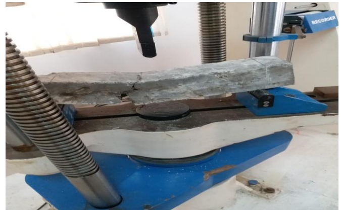
Figure 4) Flexural test of specimen
