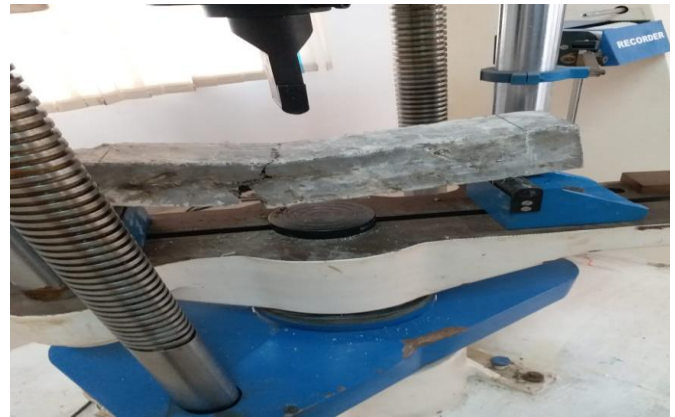
Figure 4) Flexural test of specimen
