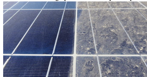
Figure 1: Clean solar panel and dust accumulated solar panel.
