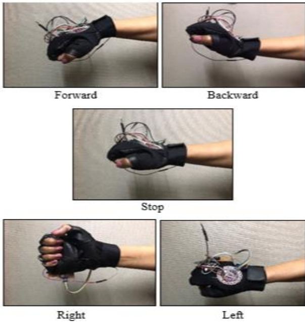
Fig. 8. Corresponding gestures to move the wheelchair
