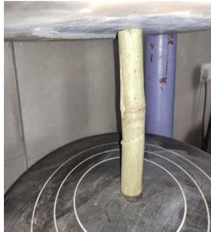
Fig. 9 Splitting failure of bamboo culm
