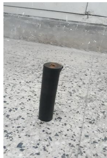
Fig. 11 PVC confined bamboo culm
