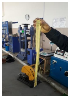
Fig. 2 Fractured sample after loading
