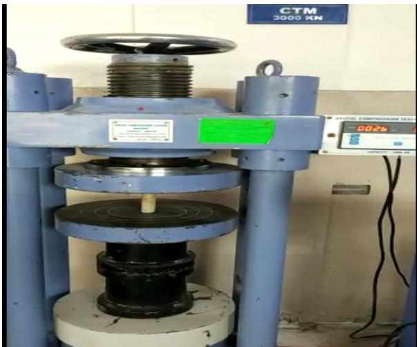
Fig.10 Compressive load is applied on sample
