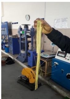
Fig. 2 Fractured sample after loading
