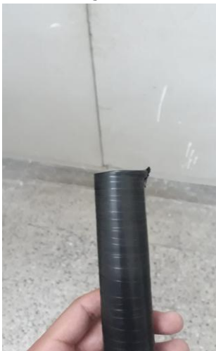
Fig. 13 End bearing failure of sample
