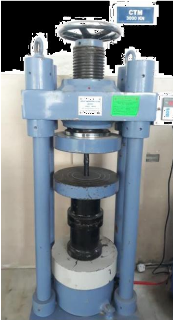
Fig.12 Applying load on PVC confined sample using UTM
