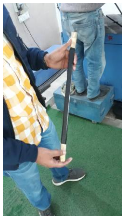
Fig. 6 Dog bone shape sample of bamboo splint
