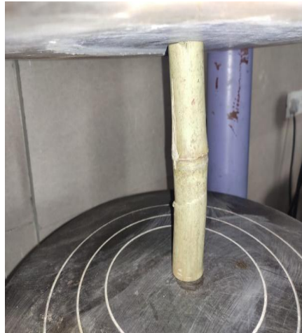
Fig. 9 Splitting failure of bamboo culm
