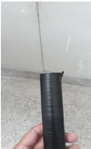
Fig. 13 End bearing failure of sample
