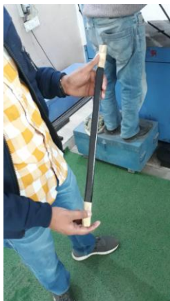
Fig. 6 Dog bone shape sample of bamboo splint
