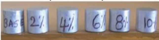
Figure 5. Cylinder-shaped specimens utilized for upset tests before deformity.
