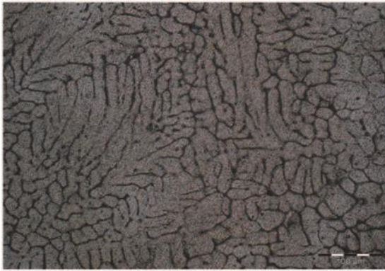
Figure 7. Optical microscopic structure of as-cast Al 6061 alloy, at 200 (scale: 100 mm) with etchant: Keller's reagent.
