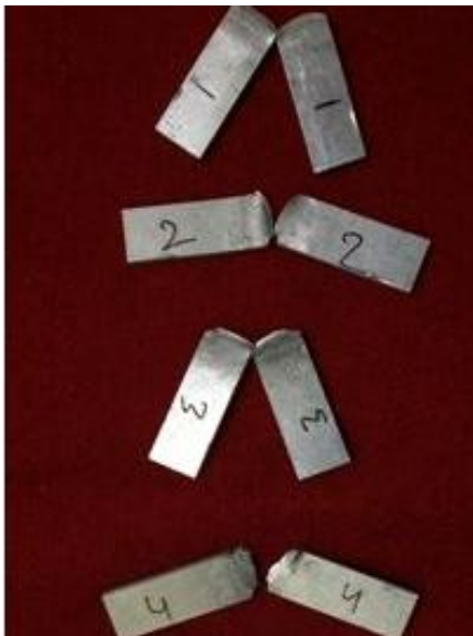
Figure 9. Impact test specimen after test
