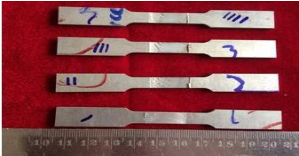
Figure 6 Tensile test specimens before test
