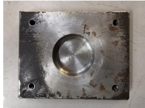
Fig 4: Die block having a cylindrical hole of the diameter of 57 mm with a corner radius of 7.5mm
