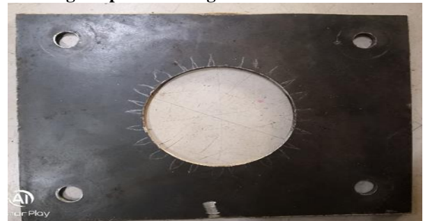
Fig7. Guide plate having a cylindrical hole of a diameter of 55mm
