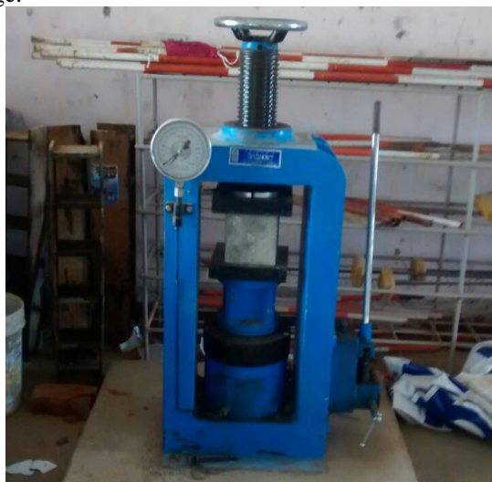
Fig. 2. Compression test on cube specimen
