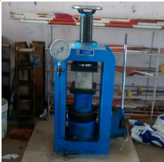
Fig. 2. Compression test on cube specimen
