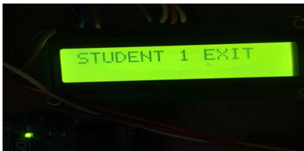
Fig. 15.LCD display when student exits the bus at College premises
