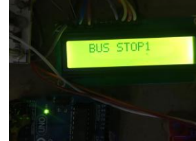
Fig. 11.LCD display when BUS STOP tag is placed on reader
