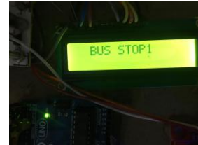
Fig. 11. LCD display when BUS STOP tag is placed on reader
