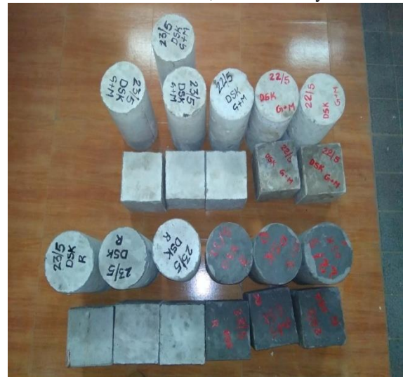
Fig (c) GPC Specimens after removing moulds
