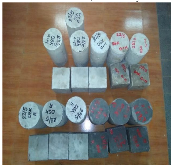
Fig (c) GPC Specimens after removing moulds
