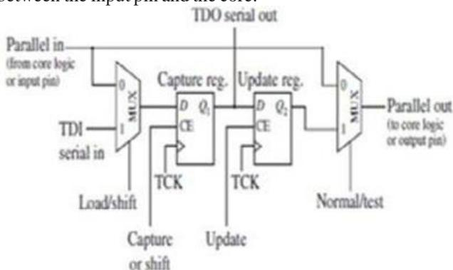
In the output side , the cells are placed between the output and the core functional pin. In normal mode , the cells just pass the data into and out of the core. In test mode , it can pass the data serially via TDI to TDO. They are used to check the pin to pad connectivity and identify where the fault occurs.
