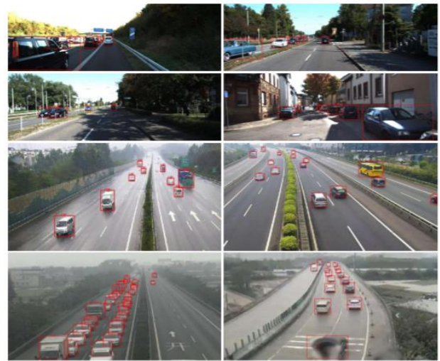
Fig-3 Example of detection results by our SINet on KITTI data set.
