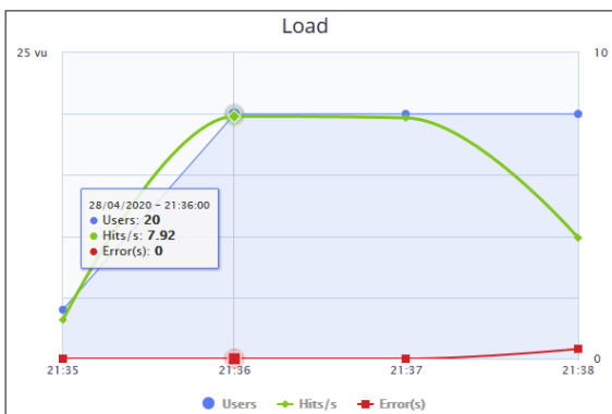
Fig. 16.Load test graph for concurrent GET request using Blazemeter tool
