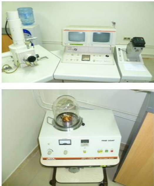
Fig. 8. The scanning electron microscope with the sputtering device used
