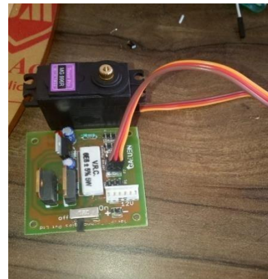
Fig 17 Servo motor with Driver IC
