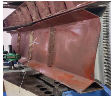
Fig.9 Failure pattern of B2
