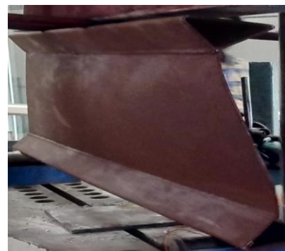
Fig.12 Failure pattern of B5
