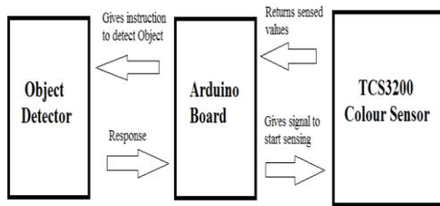
Arduino Board instructs object detector to detect the object. The sensed value from object detector is given to analog pin A5 of the Arduino. Arduino receives this sensed value and if value received at pin A5 is greater than 800, Arduino Board interprets that the object is approaching. It then instructs Colour Sensor to start sensing the object. Purpose of object detector is to reduce the consumption of colour sensor.
