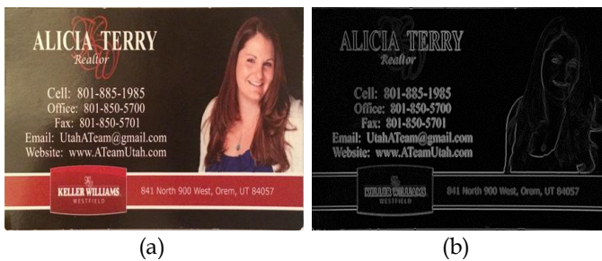
Fig. 3. Generation of morphological Gradient (a) Input image (b) Morphological Gradient image.
