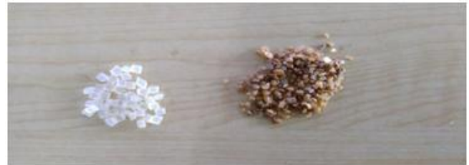
Fig. 2. Size of the filter media were used in this study. From left-handed to right-handed (HDPE granules 3.5 mm, sand media 2.5 mm).
