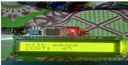
Figure 3. when a RFID tagged product is scanned and added
