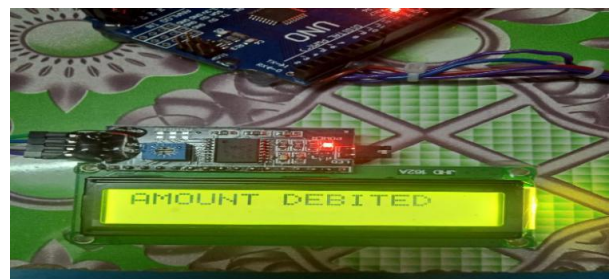
Figure 9. After pressing push button, final bill payment is done through pre-charged card.
