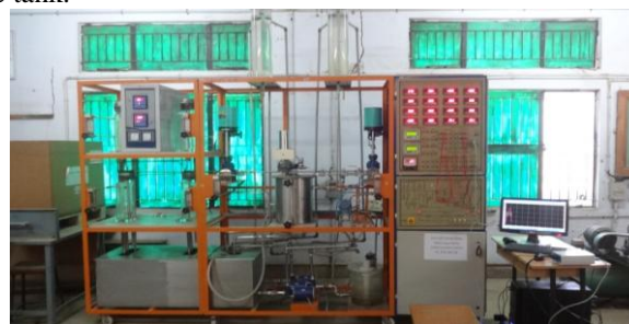
Fig. 1. Laboratory Coupled tank process
