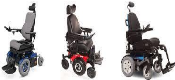
Fig (5) Different Drive wheel configuration [7]
