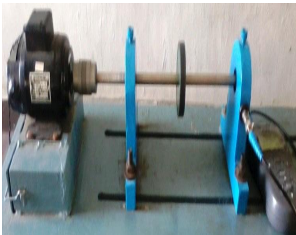
Fig 1. Experimental set up of rotor - FFT analyzer kit Taguchi analysis:
