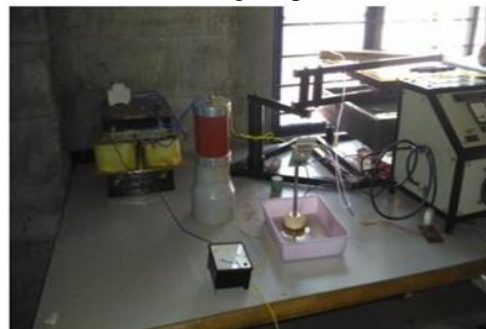
Fig. 2 Experimental Setup for Inclined Plane test
