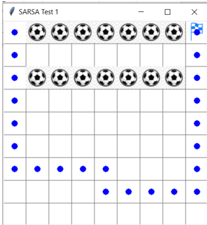
Fig. 4. One of the safe paths calculated using the SARSA algorithm with path length of 22
