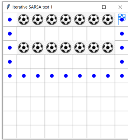
(c) Iteration 3 (from start to end) with path length 16 Fig. 6(a)(b)(c). Safe path calculated for each iteration using the Iterative SARSA algorithm
