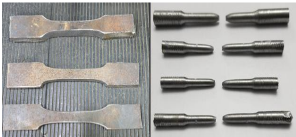
Fig. 2. Material test coupons and tested bolts
