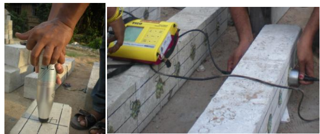
Fig. 2 Rebound hammer test Fig. 3 UPV test on columns
